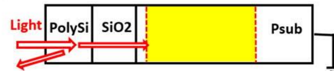
(2,3) MOS Capacitor type Photo Sensor with fairly good short wave blue light sensitivity
